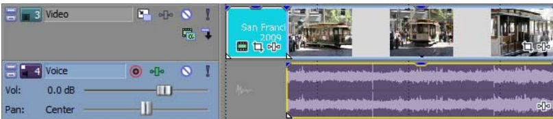
Two events that contain video (top) and audio (bottom) streams from a single multimedia video file; each event is inserted on a separate track.
