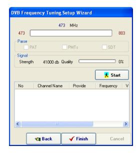
In this step, it shows the scan range and signal strength. The frequency range depends on the country where you are situated or user defined setting. The signal strength shows the terrestrial signal receiving status. When all the settings are checked, click "Start" to scan channels.
