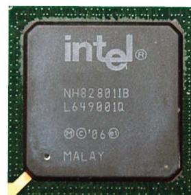
↑ ICH9R, which is paired with the P35 South Bridge chip, supports Serial ATA 3.0Gbps, External SATA interface, and RAID 0/1/5/10 functions.
