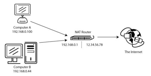
Assume a server is behind a NAT router. Imagine what happens if a client requests passive mode but the server does not know the external IP address of the NAT router. So the server sends its internal address to the client. In that case two things could happen:
